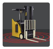
Audible alarms provide warning that a lift truck is in close or immediate proximity, and automatically self-adjusts to 5 decibels louder than the surrounding ambient noise, eliminating need for constant manual adjustments
